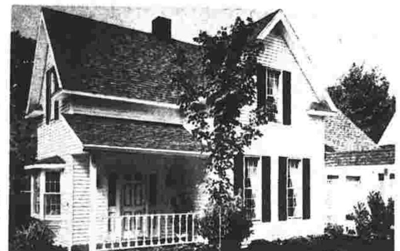
Owners created an attractive country look that's easy to maintain in the "after" photo by adding new low-maintenance siding made of Duranyl vinyl, aided by designer front door, porch posts, and lanterns. Note the relocation of the entry to make a better floorplan inside.
